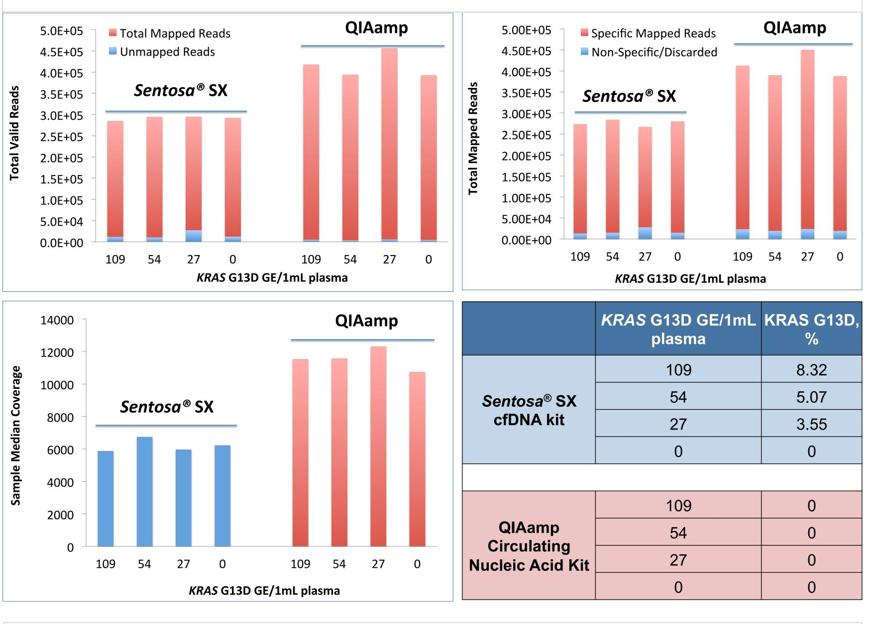
Figure 3. Assessment of cfDNA quality and quantity extracted by Sentosa<sup>®</sup> SX cfDNA Kit and QIAamp Circulating Nucleic Acid Kit using the NGS-based Sentosa<sup>®</sup> SQ CRC Panel (4x8).
